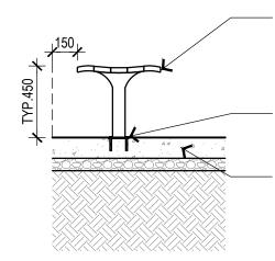
TYPICAL BENCH SEAT, PRODUCT AS NOMINATED. SLATS TO BE COMPOSITE OR STAINLESS STEEL, FRAME TO BE HOT DIP GALVANISED OR STAINLESS STEEL 316. ENSURE SLATS HAVE TAMPER-PROOF FIXINGS. SEAT IS TO COMPLY WITH AS1428.2
