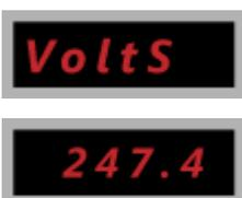
**The display shows Mains Voltage in volts (V)**
