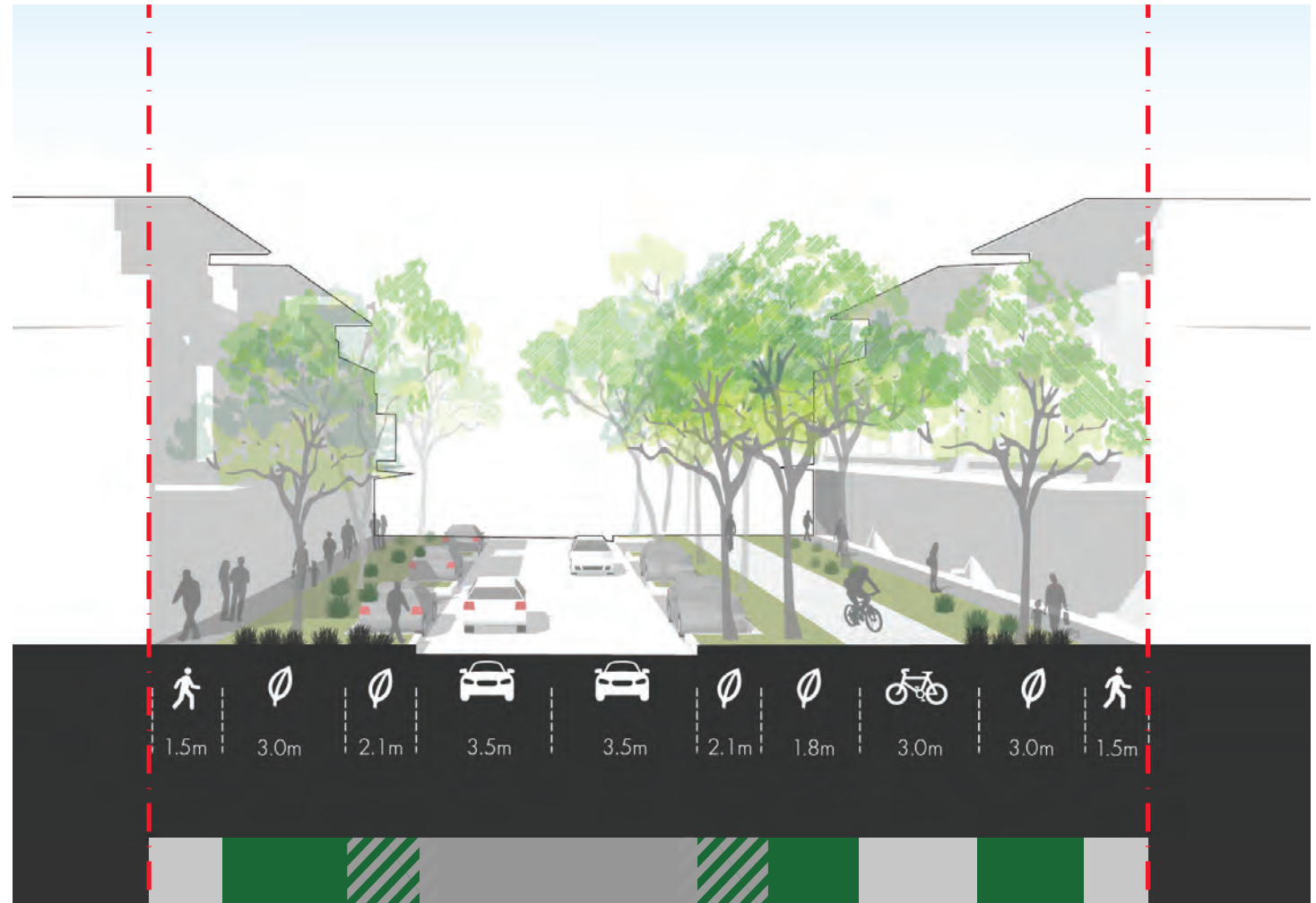
Figure 21. Connector A Section (25m)
