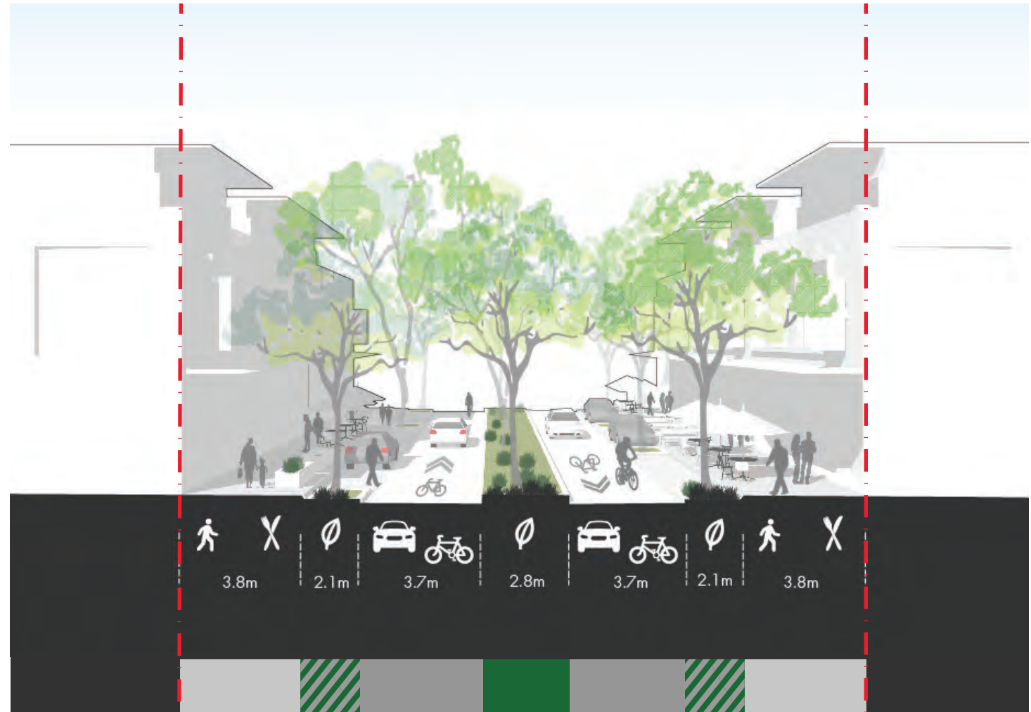
Figure 25. Urban Core Street A Section (22m)
