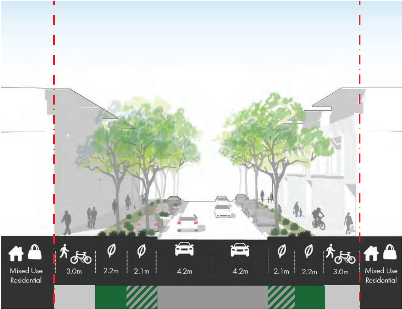
Figure 24. Connector Road C Section (23m)
