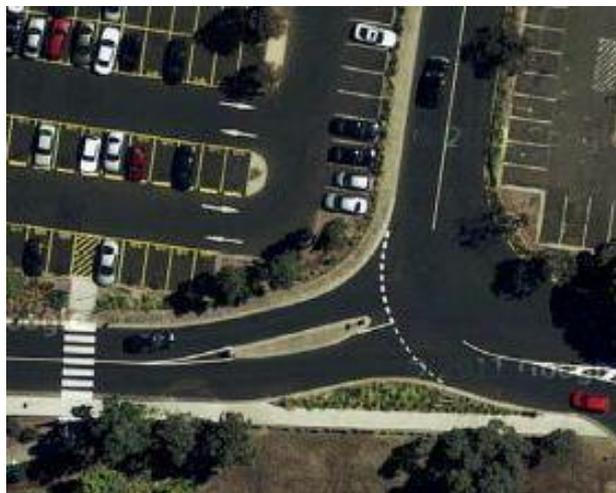
Figure 26 – Modification of T-intersection provides clear traffic priority removing ambiguity.
