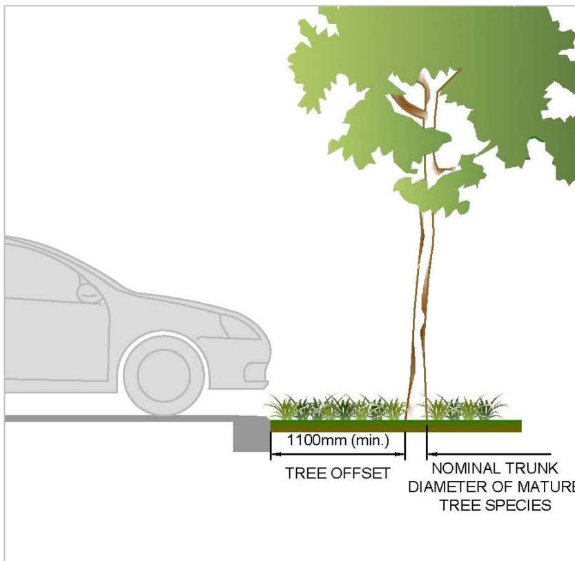
Figure 8 – Minimum vehicle (front or back) clearance to trees
