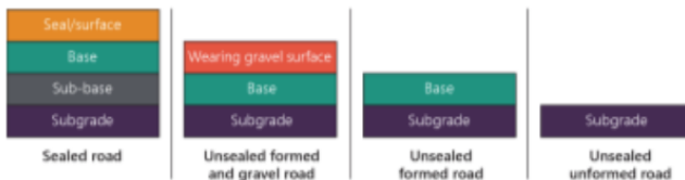
FIGURE 1C: Layers of sealed and unsealed roads
