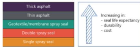
FIGURE 1D: Hierarchy of seal types based on life expectancy, durability and cost
