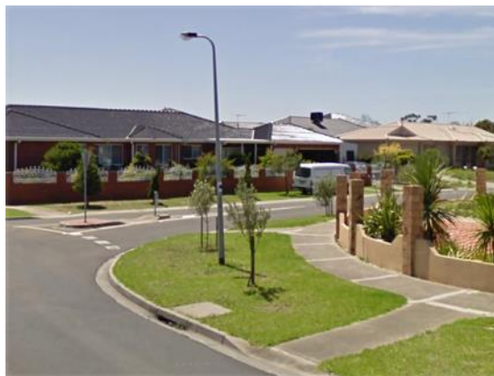
Figure 25 – Light Pole Installed Clear of Pram Crossing
