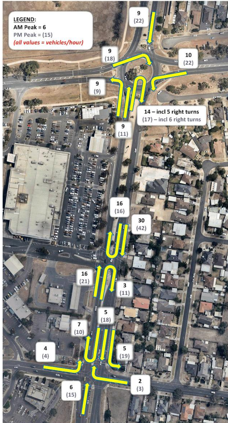
Figure 15: Traffic Volume Increases at Full Development (AM & PM peak hours) – Forecast Distribution
